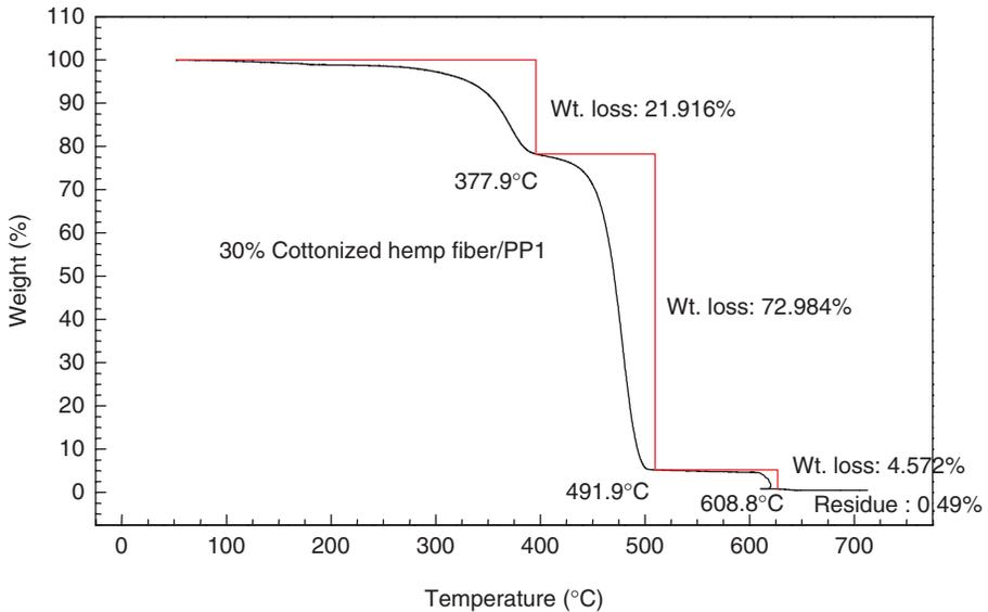
**Figure 11.** Thermogravimetric curve of 30% cottonized hemp fiber/PP1.
