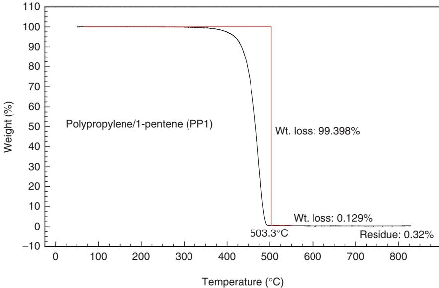
**Figure 6.** Thermogravimetric curve of polypropylene/1-pentene copolymer.
