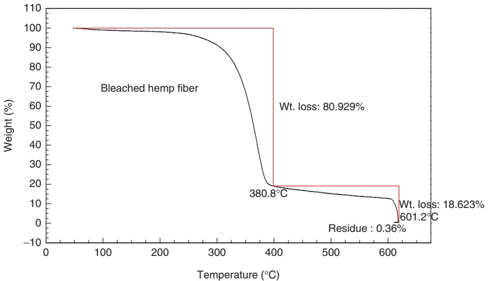
**Figure 7.** Thermogravimetric curve of bleached hemp fiber.
