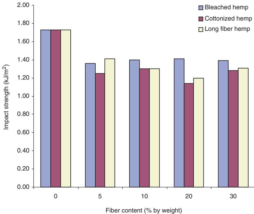
Figure 5. Effect of fiber content in PP1 on impact strength.
