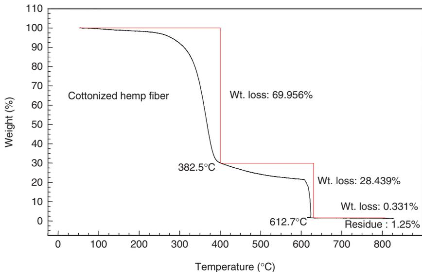
Figure 8. Thermogravimetric curve of cottonized hemp fiber.
