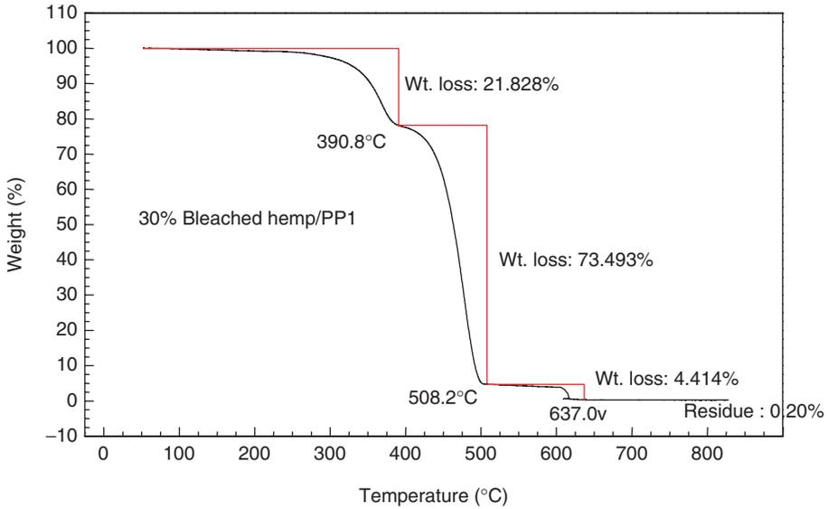
**Figure 10.** Thermogravimetric curve of 30% bleached hemp fiber/PP1.
