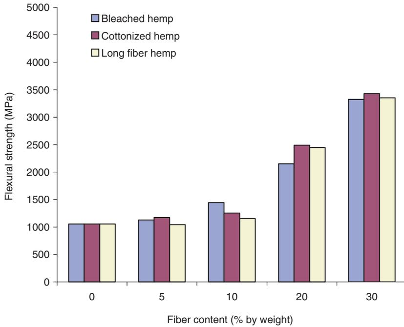
Figure 4. Effect of fiber content in PP1 on flexural strength.
