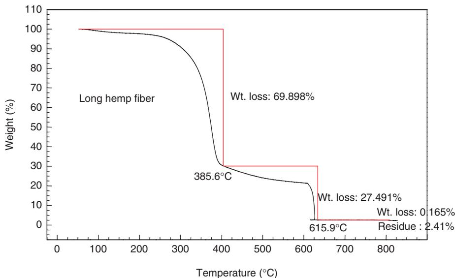
Figure 9. Thermogravimetric curve of long hemp fiber.
