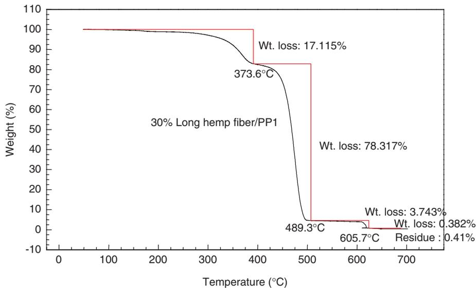
Figure 12. Thermogravimetric curve of 30% long hemp fiber/PP1.
