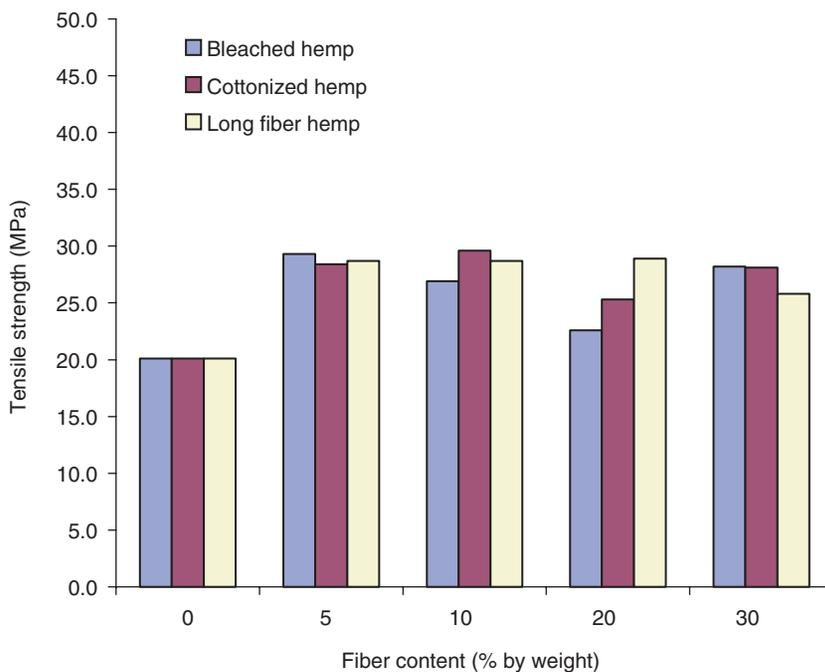
**Figure 2.** Effect of fiber content in PP1 composites on tensile strength.
