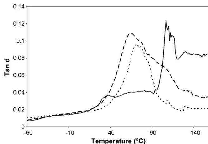
Fig. 6.  $\tan \delta$  curves of the PEG-1000-PVP mixtures: physical mixture (—); scCO<sub>2</sub>-processed (---) and ethanol-cast (· · ·).
