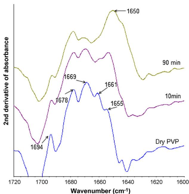
Fig. 12. 2nd derivative FTIR profiles of the carbonyl band of PVP exposed to atmospheric humidity over a period 90 min.
