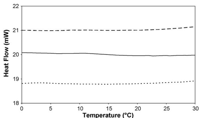
Fig. 3. DSC thermograms of the various PEG-600/PVP mixtures: physical mixture (—); scCO<sub>2</sub>-processed (---) and ethanol-cast (· · ·).
