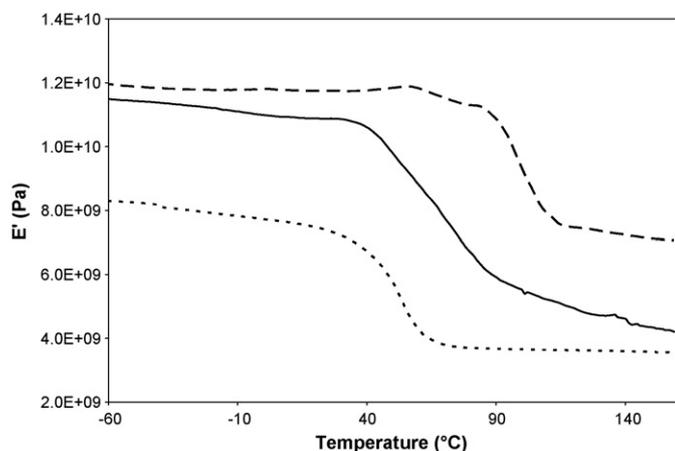
Fig. 7.  $E'$  curves of the PEG-600-PVP mixtures: physical mixture (—);  $\text{scCO}_2$ -processed (---) and ethanol-cast (· · ·).
