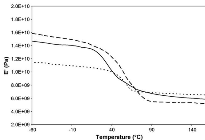
Fig. 9.  $E'$  curves of the PEG-400-PVP mixtures: physical mixture (—);  $\text{scCO}_2$ -processed (---) and ethanol-cast (· · ·).
