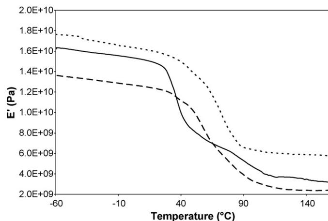
Fig. 5.  $E'$  curves of the PEG-1000-PVP mixtures: physical mixture (—); scCO<sub>2</sub>-processed (---) and ethanol-cast (· · ·).
