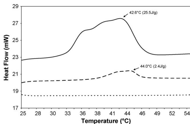
**Fig. 2.** DSC thermograms of the various PEG-1000-PVP mixtures: physical mixture (—); scCO<sub>2</sub>-processed (---) and ethanol-cast (····).
