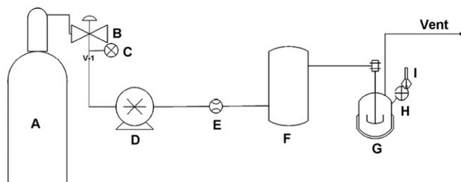
**Fig. 1.** Schematic diagram of the supercritical CO<sub>2</sub> reactor: (A) CO<sub>2</sub> cylinder, (B) back-pressure regulator, (C) pressure gauge, (D) diaphragm pump, (E) flow meter, (F) CO<sub>2</sub> pre-heater, (G) mixing chamber, (H) pressure gauge, (I) temperature probe.
