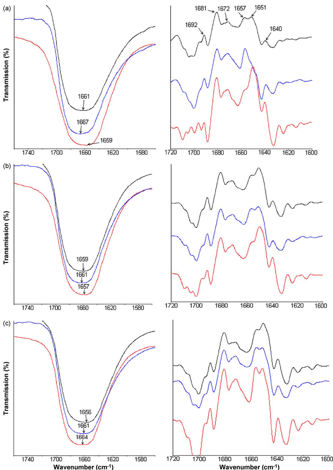
**Fig. 11.** Transmission IR spectra with corresponding second derivative spectra of the C=O region of PVP blends with PEG-1000 (a), PEG-600 (b) and PEG-400 (c) prepared by: physical mixing (—);  $\text{scCO}_2$ -processing (—); and solvent casting (—). (For interpretation of the references to colour in this figure legend, the reader is referred to the web version of the article.)
