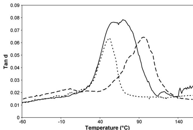
Fig. 8.  $\text{Tan } \delta$  curves of the PEG-600-PVP mixtures: physical mixture (—);  $\text{scCO}_2$ -processed (---) and ethanol-cast (· · ·).
