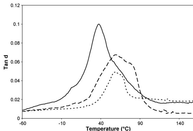
Fig. 10.  $\text{Tan } \delta$  curves of the PEG-400-PVP mixtures: physical mixture (—);  $\text{scCO}_2$ -processed (---) and ethanol-cast (· · ·).
