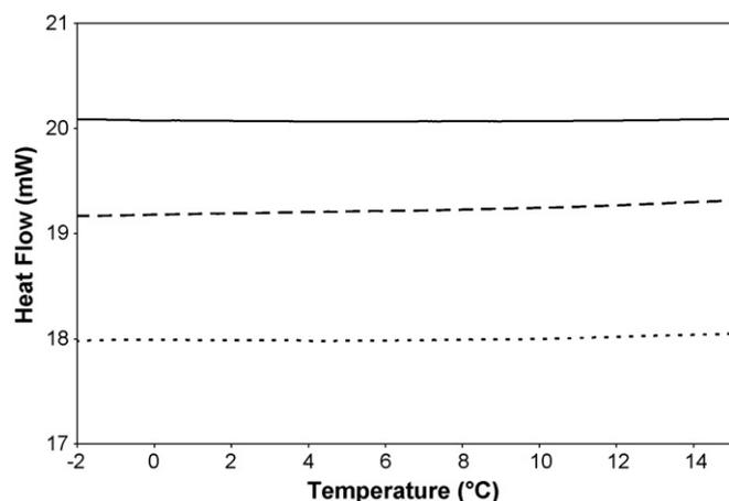
Fig. 4. DSC thermograms of the various PEG-400/PVP mixtures: physical mixture (—); scCO<sub>2</sub>-processed (---) and ethanol-cast (· · ·).
