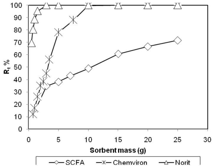
Figure 2: Effect of sorbent mass on removal efficiency (Temp 298 K; Initial concentration 5930 mg/ ℓ; Initial pH 7)
