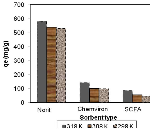
Figure 4: Effect of temperature on sorption capacity (Initial concentration: 5930 mg/ ℓ; Sorbent mass 1 g; pH 7)
