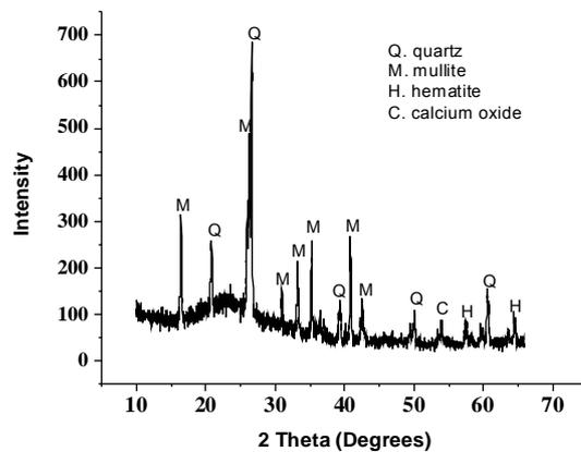
Figure 1: XRD pattern for coal fly ash
