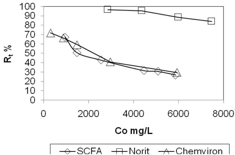
Figure 3 : Effect of initial concentration of solution on decolourization efficiency (Temp 298 K; Sorbent masses, 3 g Chemviron, 1 g Norit, 5 g SCFA; pH 7)
