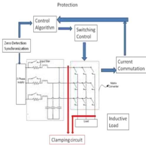
Fig. 2 – Subsystems of a Matrix Converter
