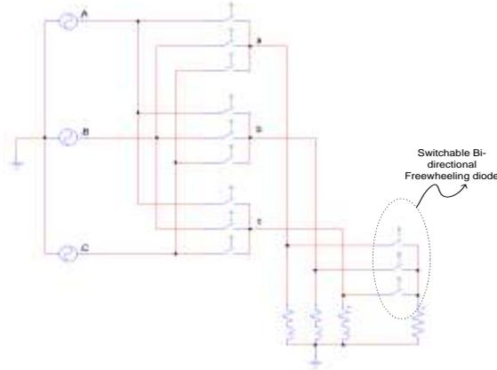
Fig. 8 – Switchable Freewheeling path
