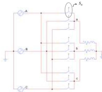
Fig. 1 – Matrix Converter
