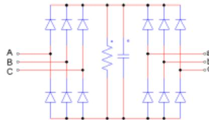
Fig. 4 – Voltage Clamp Circuit
