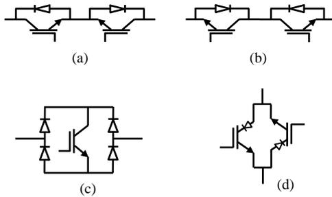
Fig. 3 – Discrete Switch layout
