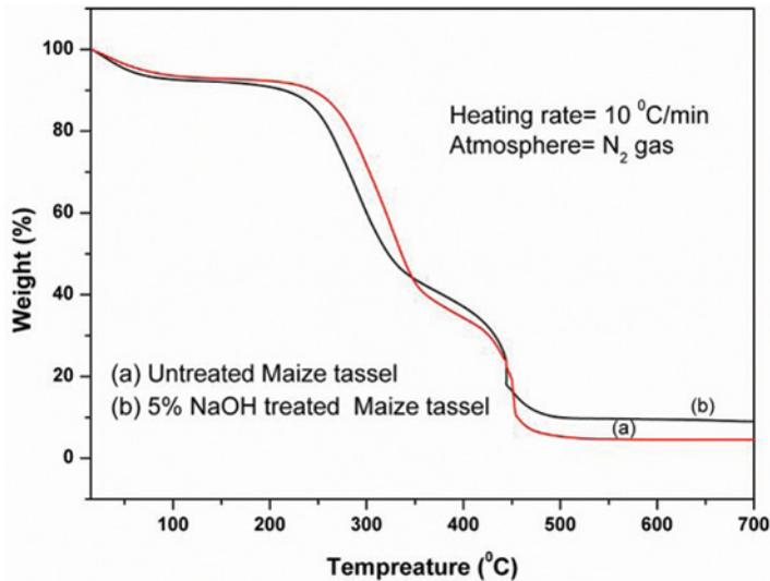
FIGURE 5 TGA thermograms of (a) untreated and (b) alkali-treated (NaOH) maize tassel fibers.
