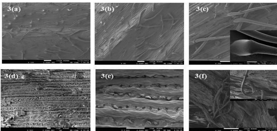
FIGURE 3 SEM micrographs of untreated and alkali-treated maize tassel fiber: (a)–(c) untreated, (d)–(f) alkali-treated (NaOH) fibers at different magnifications.
