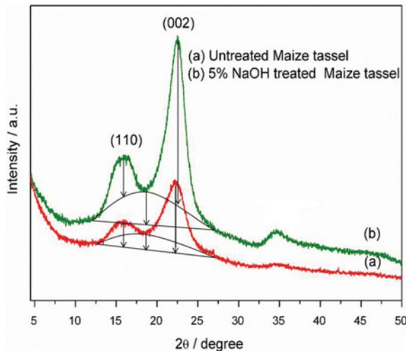
FIGURE 4 X-ray diffraction patterns of (a) untreated and (b) alkali-treated (NaOH) maize tassel fibers.
