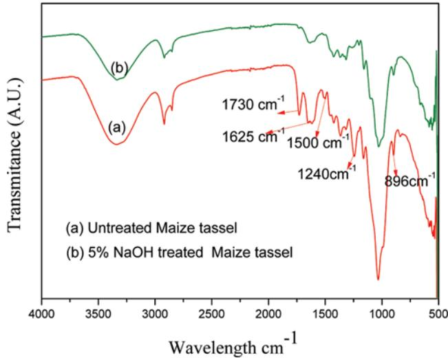
FIGURE 2 FT-IR spectra of maize tassel fiber: spectrum (a) untreated and (b) alkali-treated (NaOH) maize tassel fibers.
