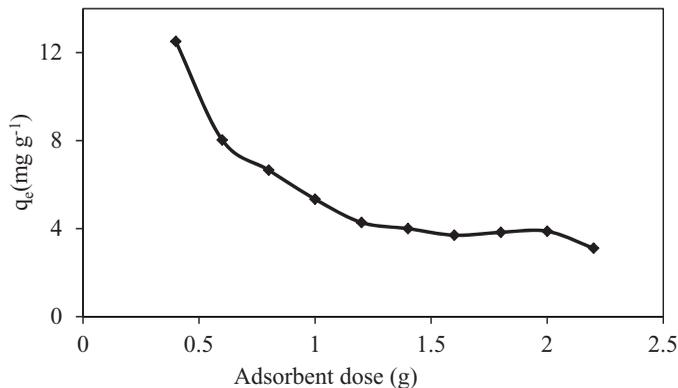
Figure 4. Effects of adsorbent dosage on the adsorption capacity of Rooibos shoots.
