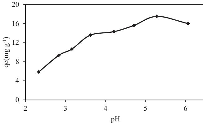
Figure 3. Effects of pH on the adsorption capacity of Rooibos shoots.
