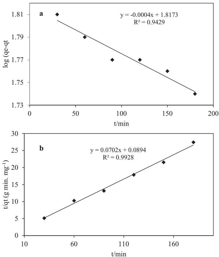
Figure 7. Pseudo-first-order plot (a) and pseudo-second-order plot (b) for cadmium adsorption onto Rooibos shoots.
