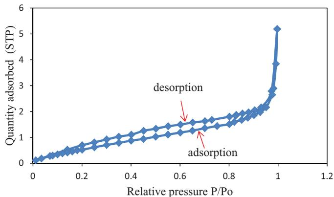
Figure 1. The nitrogen adsorption–desorption isotherm of the adsorbent prepared from Rooibos shoots.
