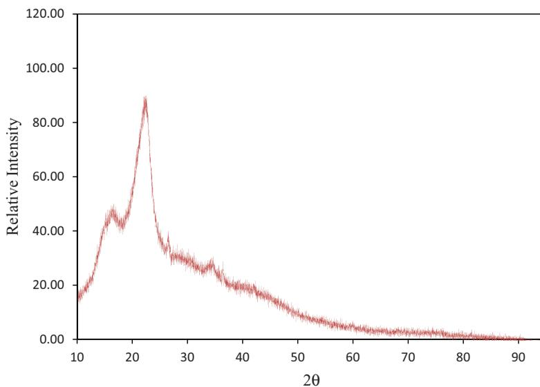
Figure 2. X-ray diffraction spectrum of Rooibos shoots.
