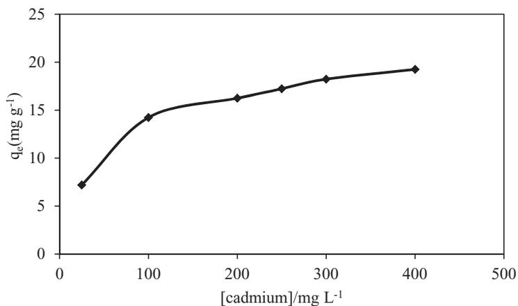
Figure 5. Effect of initial cadmium concentration on adsorption capacity of Rooibos shoots.
