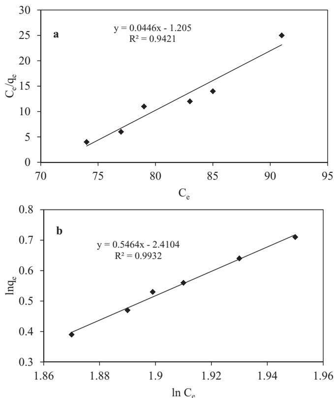
Figure 8. Langmuir isotherm (a) and Freundlich isotherm (b) for cadmium adsorption onto Rooibos shoots.
