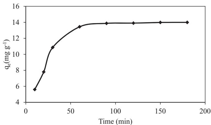
Figure 6. Effect of contact time on adsorption capacity of Rooibos shoots.
