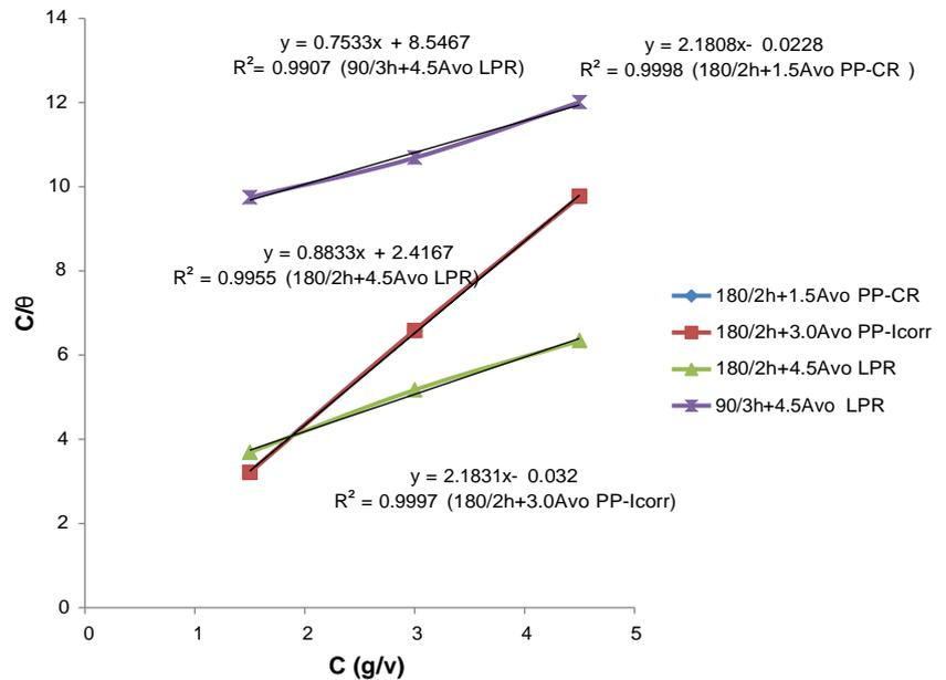
by this inhibitor increased. Hence, IE was enhanced significantly. It can be seen that the alloy with conventional thermal treatment demonstrated better corrosion resistance than those pre-aged prior to thermal treatment. From this behaviour, coupled with simultaneous change in the anodic and cathodic region during the electrochemical measurement Avogadro oil can be said to exhibit a mixed-type corrosion inhibition. This occurrence agrees with previous reports [12, 14].
