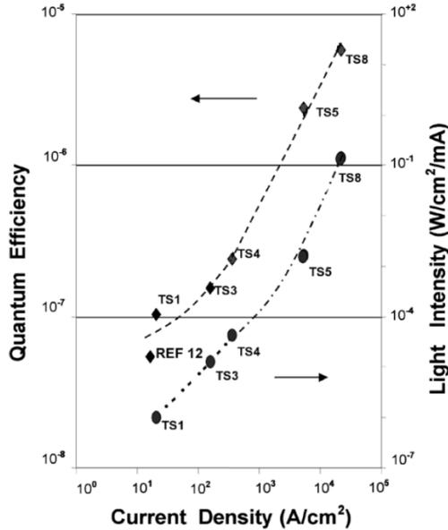
Fig. 4. Calculated normalized quantum efficiencies and measured light intensity as a function of current density through the active light-emitting areas of the devices for various silicon CMOS light-emitting test structures that operate in the reverse bias avalanche mode of operation.
