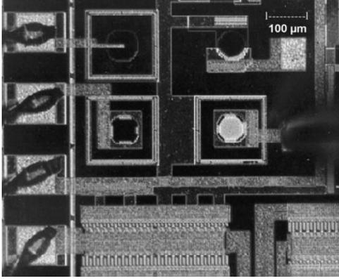
Fig. 1. Photomicrograph of a 60- $\mu\text{m}$ -diameter optical fiber interface (TS4) as realized with 1.2- $\mu\text{m}$  bi-CMOS technology. The light emission level is  $\sim 4 \times 10^{-4} \text{ W} \cdot \text{cm}^{-2}$  or about 1 nW for the area shown.
