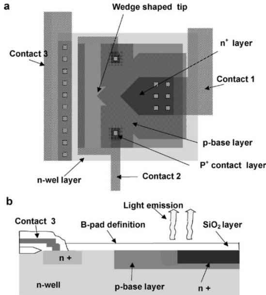
Fig. 2. Schematic planar layout and cross-sectional layout of shallow-junction planar  $n^+ pp^+$  Si light emitting device using a 2- $\mu\text{m}$  silicon CMOS technology with a bipolar capability.
