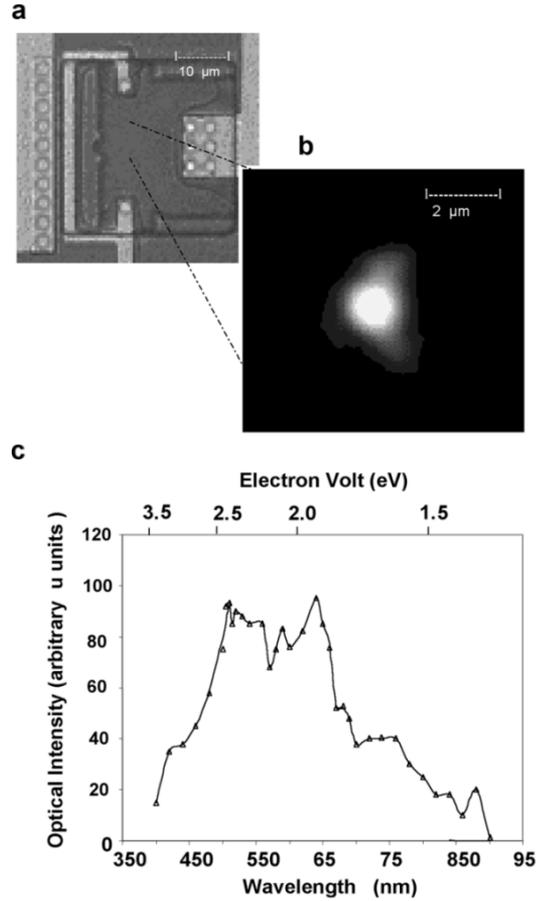
Fig. 3. (a) Photomicrograph of test structure 8 (TS8) and shallow-junction planar  $n^+ pp^+$  Si light-emitting device using a 2- $\mu\text{m}$  silicon CMOS technology with a bipolar capability. (b) Performance characteristics of the device under subdued ambient lighting conditions at 8 V and 0.1 mA. (c) Spectrographic data for the TS8-type structures.
