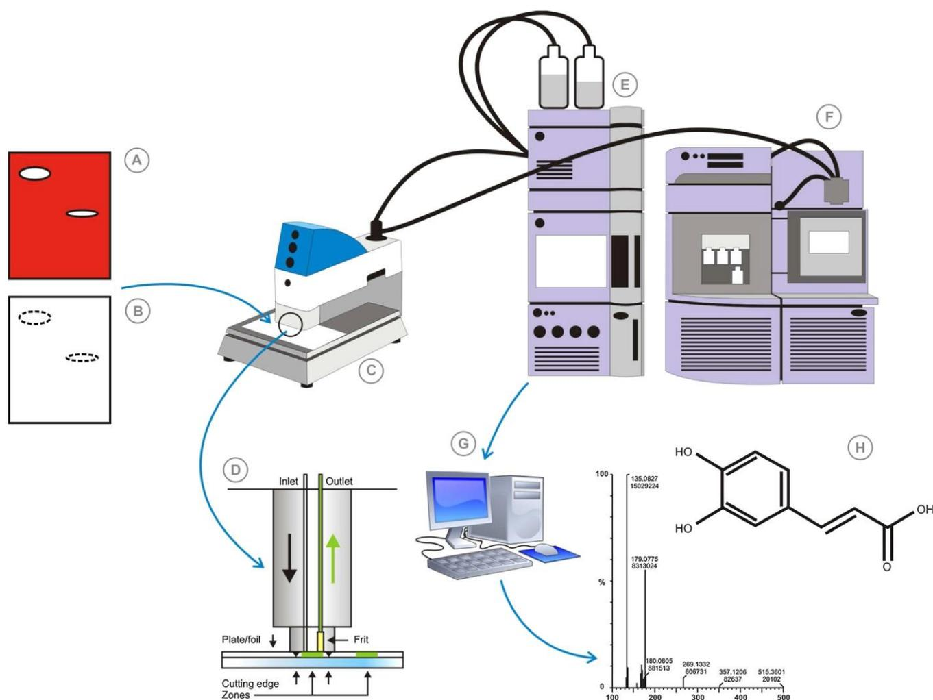
Fig. 1. Workflow diagram illustrating the hyphenated high performance thin layer chromatography-bioautography-mass spectrometry (HPTLC-bioautography-MS) technique used to identify antimicrobial compounds in propolis. (A) Bioautography HPTLC plate, (B) reference HPTLC plate, (C) TLC interface, (D) flowpump enabling the elution of target compounds from the plate, (E) UPLC pump, (F) time-of-flight mass spectrometer, (G) data analysis, and (H) mass spectral data allowing identification of compounds.
