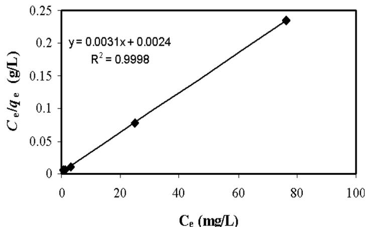
**Figure 9.** Linearized Langmuir isotherm (Equation 4) for Pb(II) adsorption onto HT nanoparticles at 298K.
