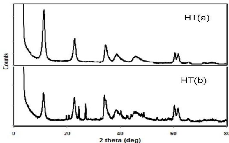
**Figure 4.** XRD analysis of the HT nanoparticles before (a) and after  $\text{Pb(II)}$  adsorption (b).
