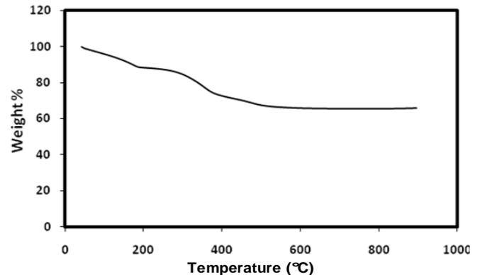
**Figure 2.** Thermogravimetric analysis of the HT nanoparticles.
