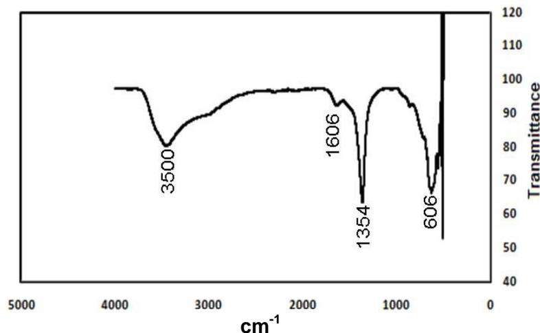
**Figure 3.** FTIR spectra of the HT nanoparticles.
