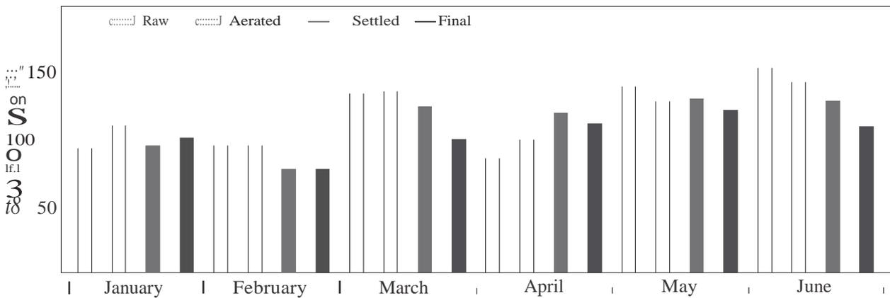
**Figure 5:** Total solids in the raw water, after aeration, sedimentation, filtration and disinfection
