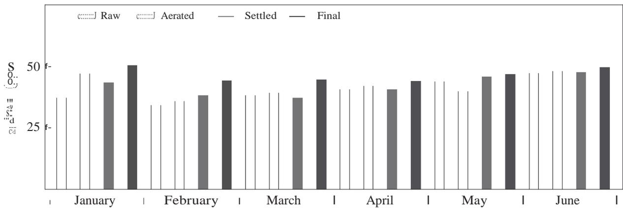
**Figure 6:** Variation of total hardness in the raw, aerated, settled and treated water
