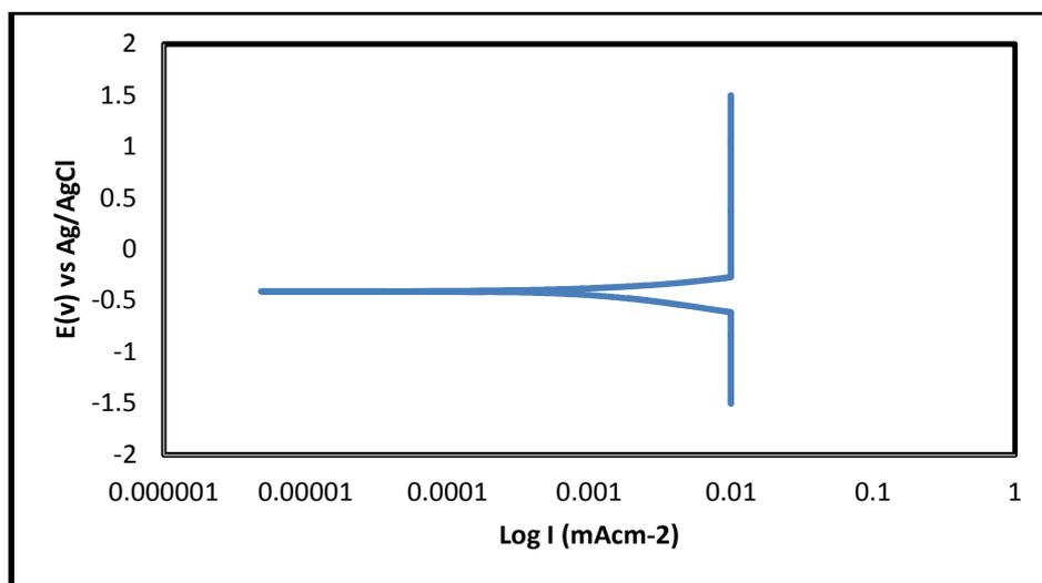
Figure 9: Polarization curve of mild steel in HCL
