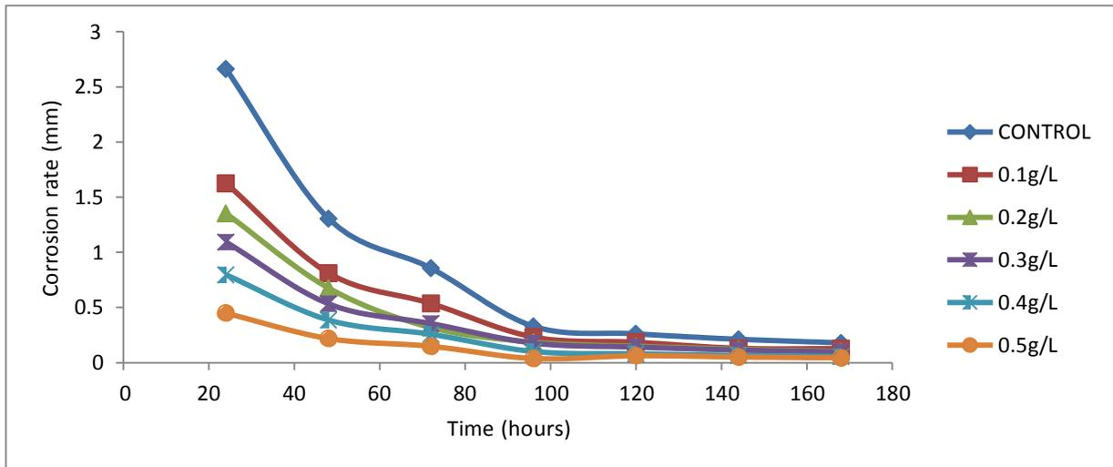
Figure 3: Corrosion rates of aluminium in 3.5% NaCl at 304K at different inhibitor concentration
