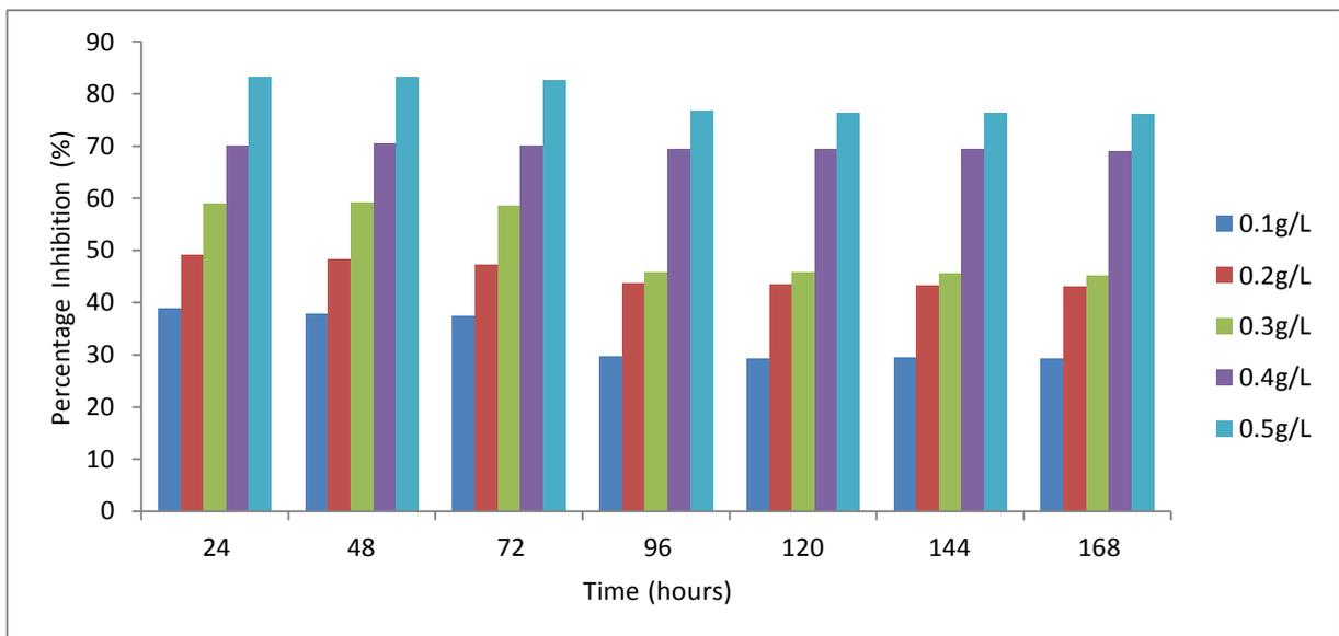
Figure 4: Percentage inhibition efficiency of aluminium in 3.5% NaCl at 304K at different inhibitor concentration
