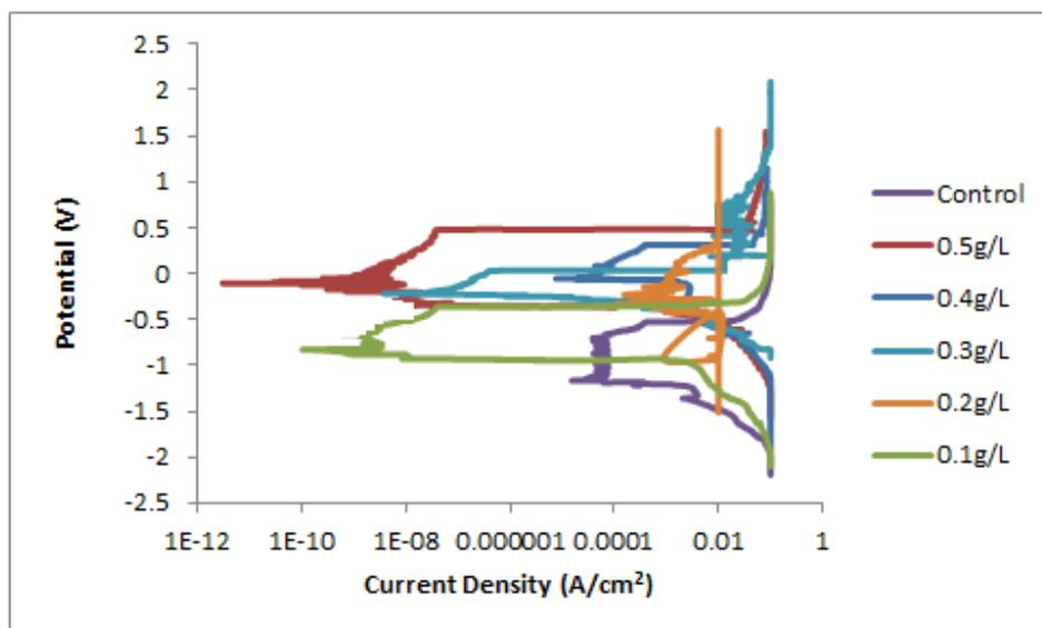
Figure 5. Tafel polarization curves of aluminium alloy in 3.5% NaCl solution in the absence and presence of different concentrations of silicone oil
