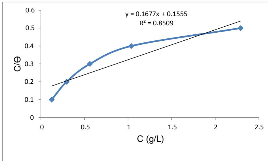
Figure 6. Langmuir adsorption isotherm model for silicone oil in 3.5% NaCl medium
