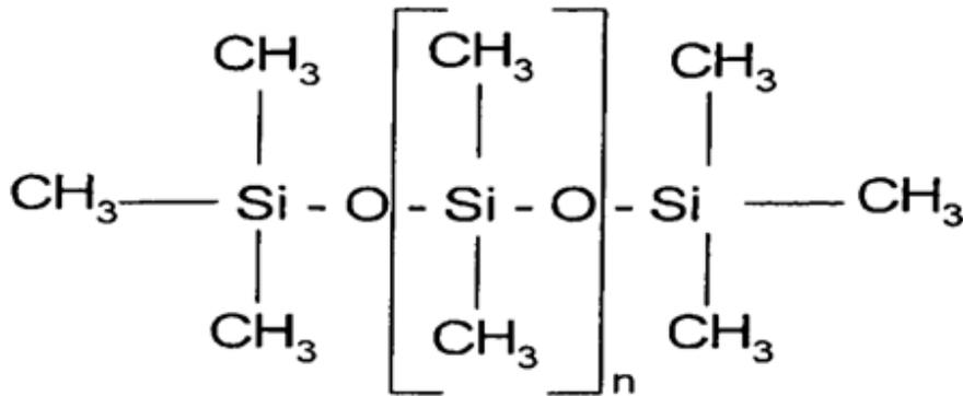
Figure 1. Molecular structure of silicone oil
