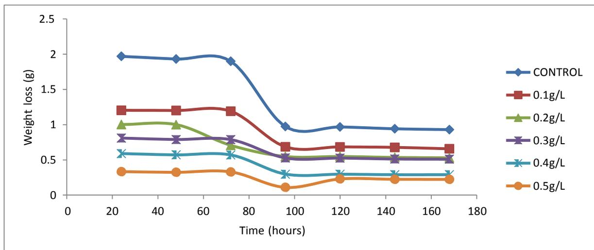
Figure 2: Weight loss of aluminium alloy with time of immersion in 3.5% NaCl at 304K at different inhibitor concentration
