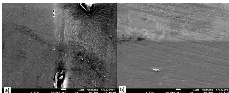
Figure 3: SEM micrographs of the cross-sectional view of 95Ti-5SiAlON coatings deposited at scan speed a) 0,6m/min and 1,2m/min captured at the coating/substrate interface
