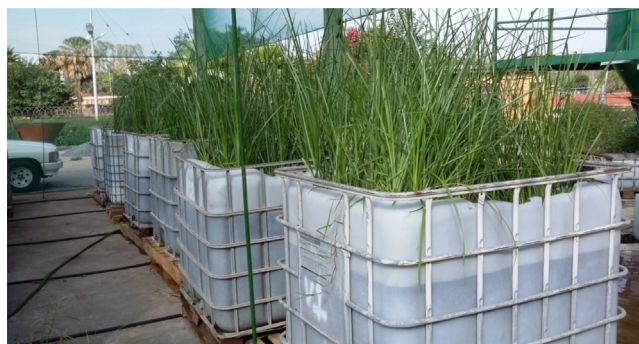
Fig. 1. Experimental setup showing a section of the pilot VSBCW with V. Zizanioides .
