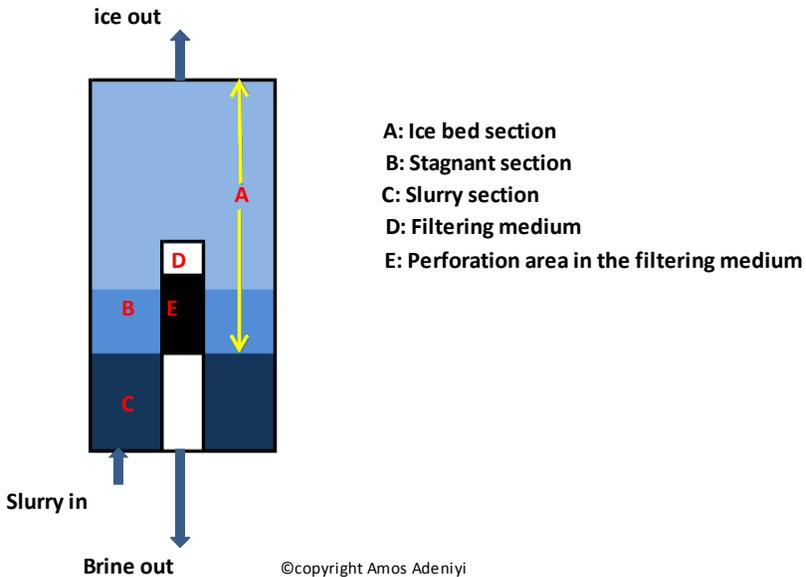
Figure 3: Sections in the HybridICE HIF filter.
