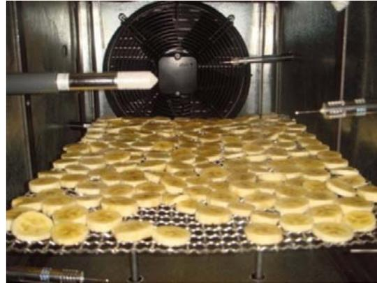
**Figure 6:** Batch type dryer, inside view with sensors
