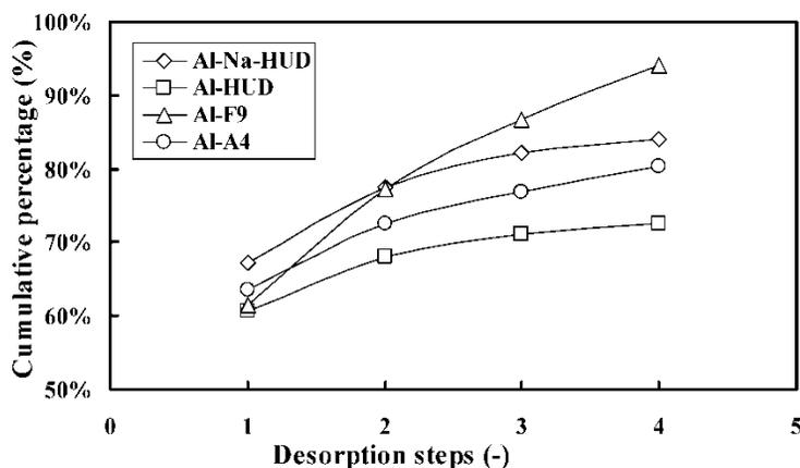
**Figure 11.** Desorption of fluoride from  $\text{Al}^{3+}$ -pretreated low-silica zeolites using sodium bicarbonate as a desorbing agent.
