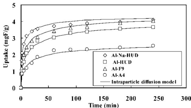
**Figure 9.** Effect of zeolite type on the uptake of fluoride at various time values (solid lines indicate intraparticle diffusion modeling). Initial fluoride concentration = 10 mg/L, adsorbent dose = 2 g/L, agitation speed 300 rpm.
