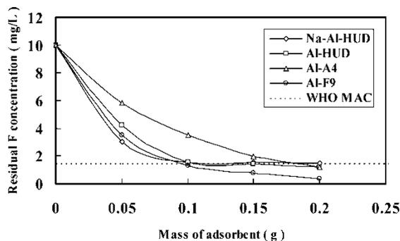
Figure 2. Effect of adsorbent mass on fluoride uptake.
