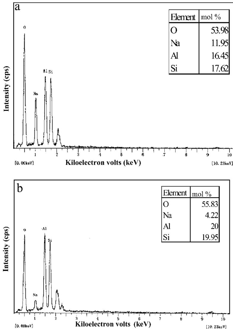
**Figure 1.** Energy dispersive X-ray spectrometry (EDXS) spectra of (a) A4 zeolite; (b) Al<sup>3+</sup>-pretreated A4 zeolite (Al-A4).
