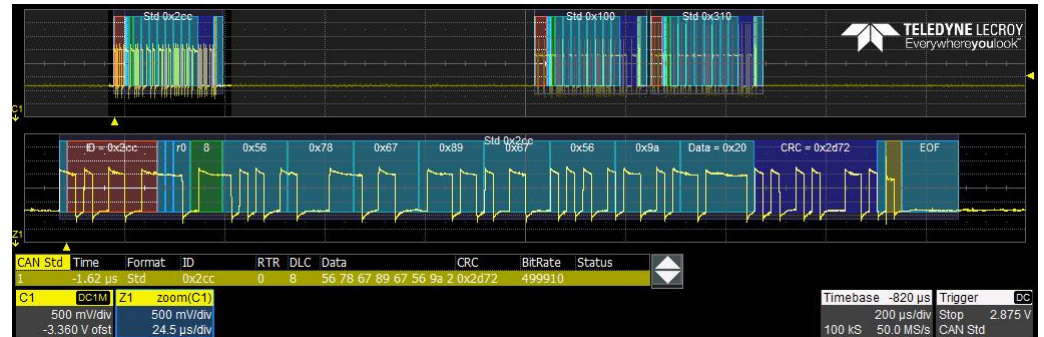
Figure 12. LECROY-bus-analyzer-captured CAN message frame.
