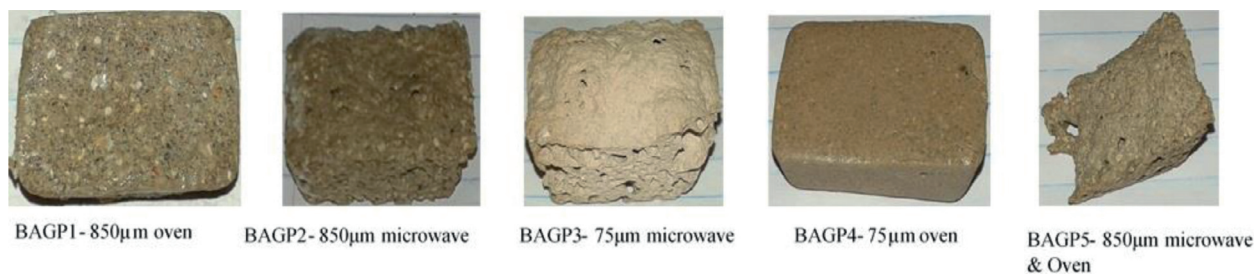
Fig. 4. Geopolymer samples used for compressive strength test.
