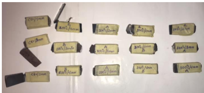
Fig. 4: V-notched AISI 1035 samples with varying thickness
