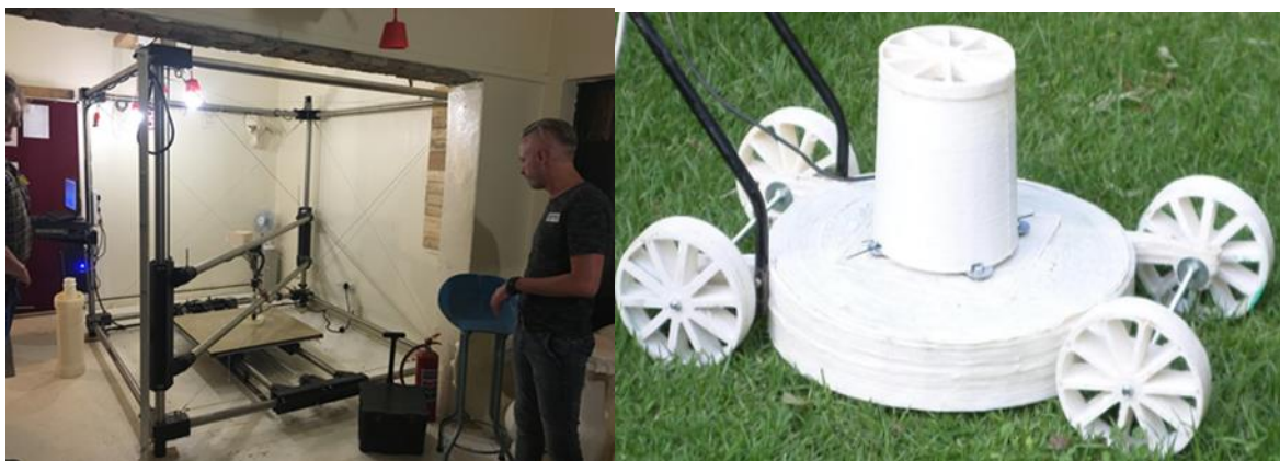
Figure 4.2: The ‘Cheetah’ and the lawn mower printed by it; Source: O Maselwanyane (2017) and Interviewee 53dprinting.com.
