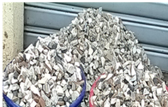
Fig. 1b Ceramic aggregates after crushing and grading.
