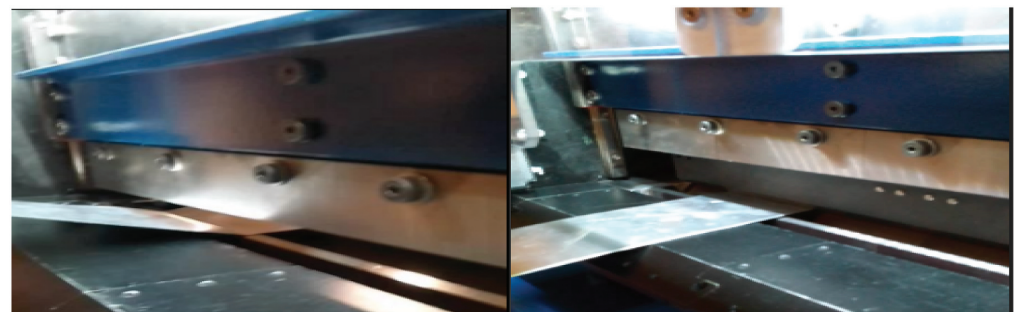
a: Cutting operation of aluminium sheet
