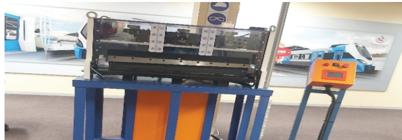
Figure 2. The reconfigurable guillotine shear and bending press machine for cutting and bending operations.
