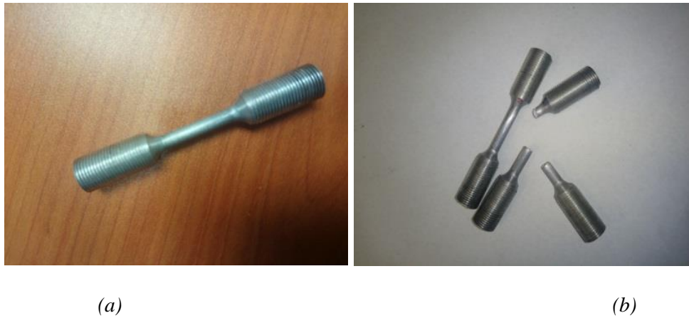
Figure 3: (a) Dog-bone sample used for axial fatigue tests (b) Fractured fatigue samples after testing.
