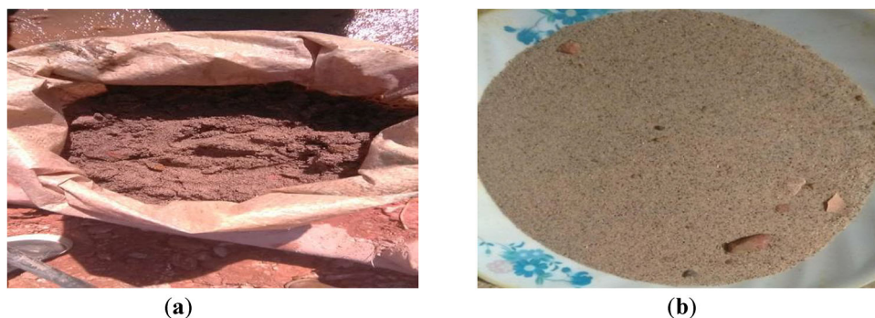
Fig. 1. Rayfield–Jos ASBCM: (a) bag of as-received sample (25 kg), (b) washed and dried sample.
